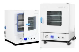
Vacuum ovens are ideally suited for baking, drying, or disinfecting various products in vacuum conditions providing faster drying since liquids evaporate at temperatures below their boiling points.
